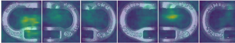
Fig. 4: Examples of spurious anomaly maps of defect samples using the masked dataset of coupling links (increased gamma and contrast).
